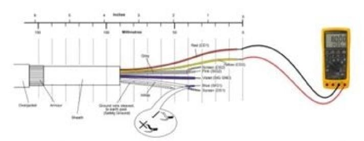
This result should be between  $5 - 100\Omega$ . Any value above or below this range is a FAIL. A fail indicates that the coil is open or short circuit. This will mean replacing the flow tube.
