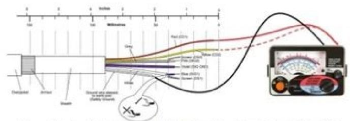
The results should be between 5 - 200MΩ. Anything below this is a FAIL. A fail indicates that the coil is shorted circuited to earth. This will mean replacing the flow tube.
